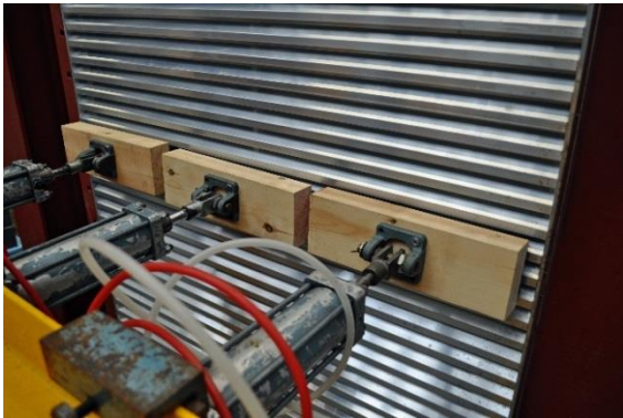
Photograph 10 Showing the application of the line load
